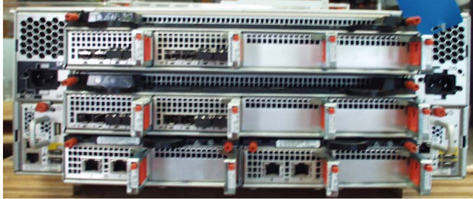
Figure 3. CX4 Model 960 storage processor and I/O annex area
