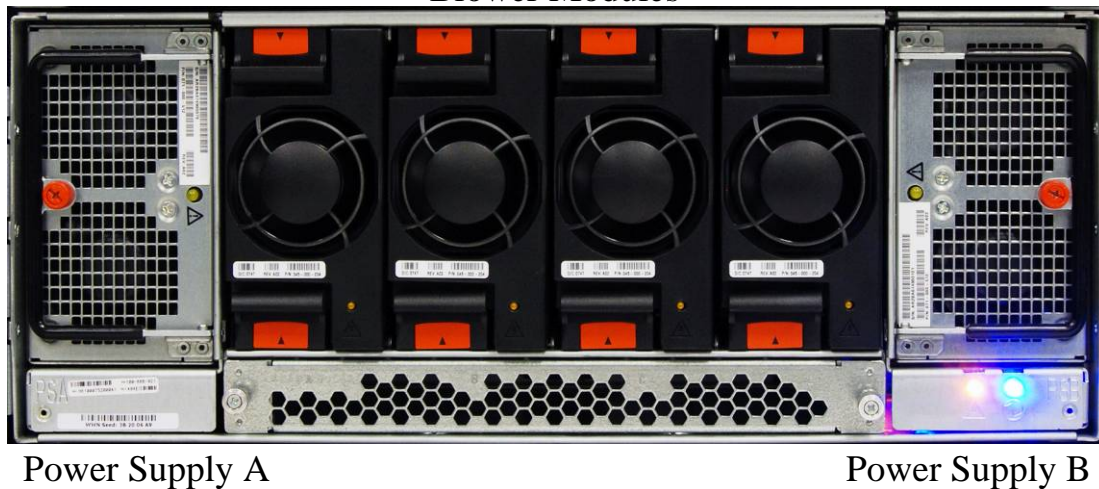
Figure 6. CX4 Model 960 power supplies and cooling
