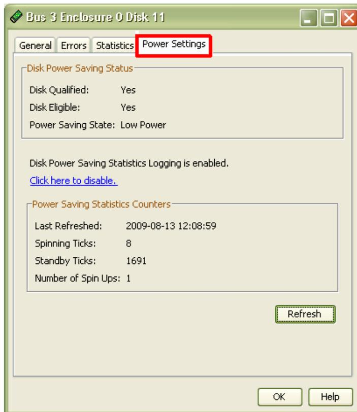
**Figure 6. Bus Enclosure dialog box: Displaying spin-down information at the disk level**
